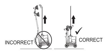
■ When transporting the GloBug 4-Spot, lower the mast fully. Tighten the lamp adjustment lever and make sure that the lighting unit assembly is fixed to the mast before transporting. This will prevent the light assembly from falling down or being damaged during transport.
